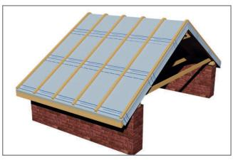
Fig 8.3.2 The counter battens
