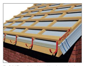
Fig 8.4.1 The oof sheathing with  $% \left( 1\right) =\left( 1\right) \left( 1\right) +\left( 1\right) \left( 1\right)$  rainwater hooks
