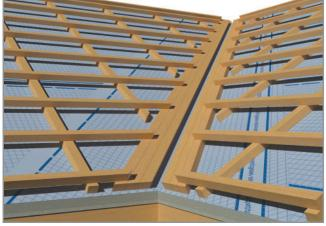
Fig 8.6.2 The batten of the valley node
