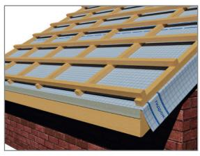
Fig 8.4.2 The roof sheathing without rainwater hooks
