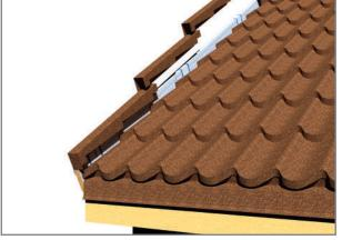
Fig 9.4.2 Gable flashing installation
