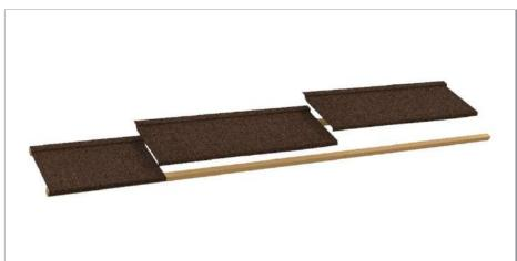
Fig 9.1.6 Overlapping the tiles from left to right
