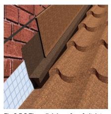
Fig 9.5.8 The adjoining of roof pitch to the wall parallel to the slope
