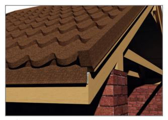
There is a need to close a protruding end. Example. Cut 4 corners from the scraps of the material. Attach them to the edge of the gable board. Then. Cut a rectangle out of a flat sheet with sides that are 2 mm smaller than the inner cavity of the board. Fasten by the riveted rivets or the screws. Treat it by the maintenance kit.
