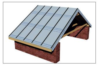
Fig 8.3.1 The tape gumming underneath the counter batten
