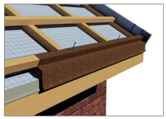
Fig 9.1.1 Small eave flashing installation
