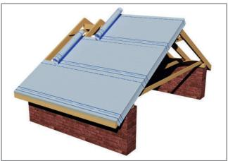
Fig 8.2 Eaves protection flashing
