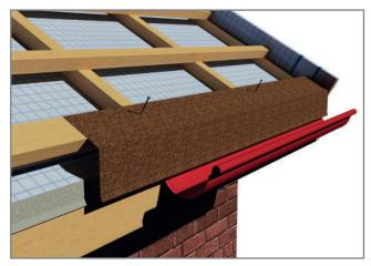
Fig 9.1.2 Big eave flashing installation
